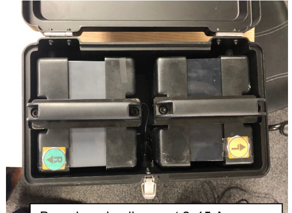
Draagbare laadbox met 2x15 Amp accu's.
